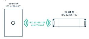
104 + 101 Bridge mode is enabled after the device has been added to a 104 controller and a 101 power supply has been connected to the DALI terminals.
